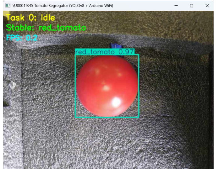
Fig. 3. YOLOv8 detection output identifying a red tomato with 97% confidence during real-time inference.
